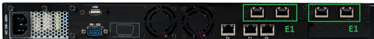
Model with 4 RJ45 connectors for 4 E1/T1 links
