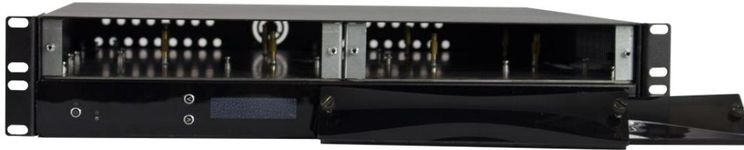
Open front view for changing SIM cards
